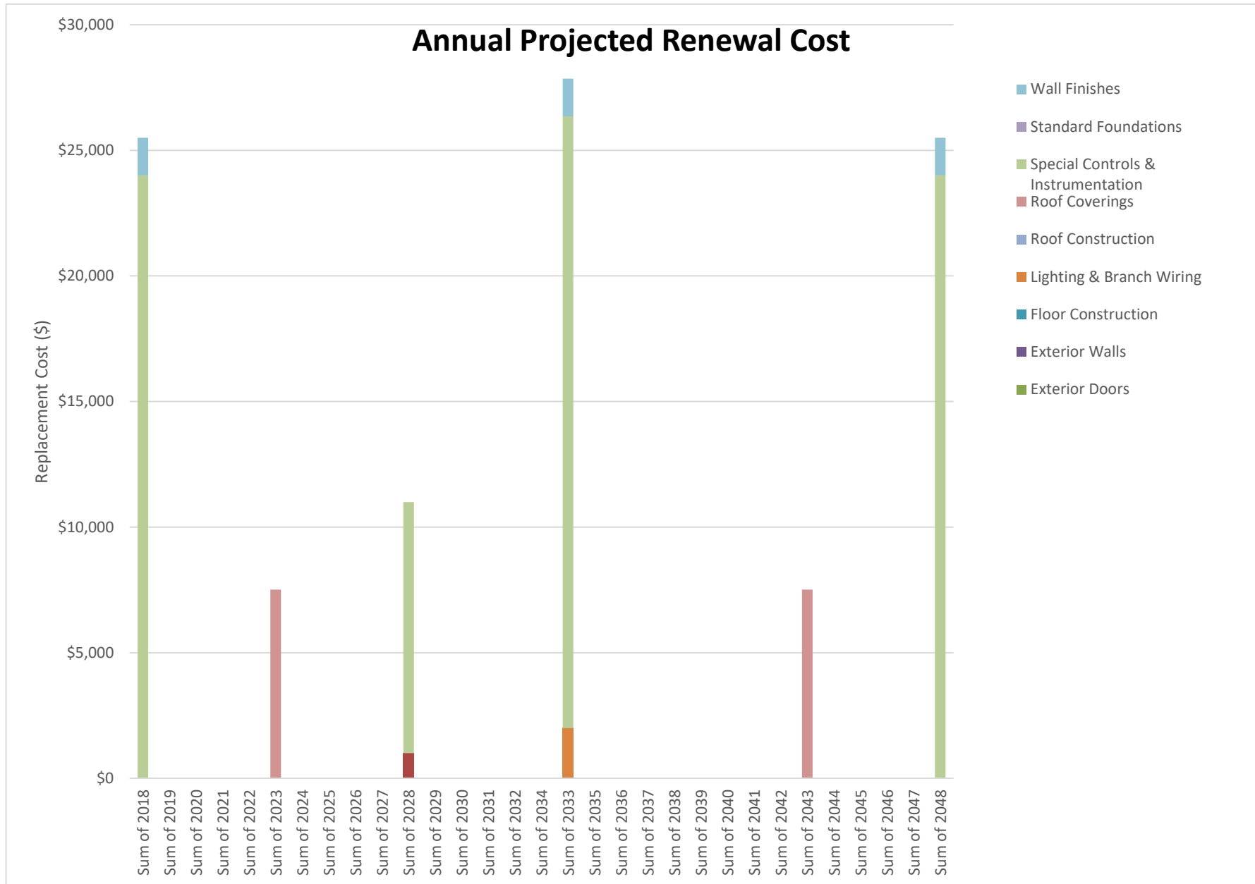
Figure 17: Annual Projected Renewal Costs for Sewer Lift Station
